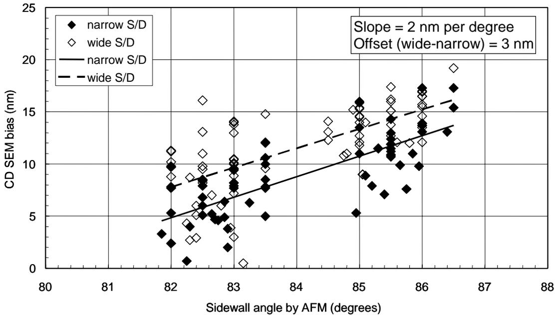
Fig. 3. Sample-to-sample CD SEM bias dependence on polysilicon line sidewall angle. The “narrow” and “wide” source and drain transistor cases stand for less than  $0.5 \mu\text{m}$  and more than  $1 \mu\text{m}$  proximity of the line to STI, respectively. CD SEM bias is defined as a difference between mid-derivative line CD by SEM and CD by AFM at 10% of the line height. Sidewall angle is measured by AFM.
