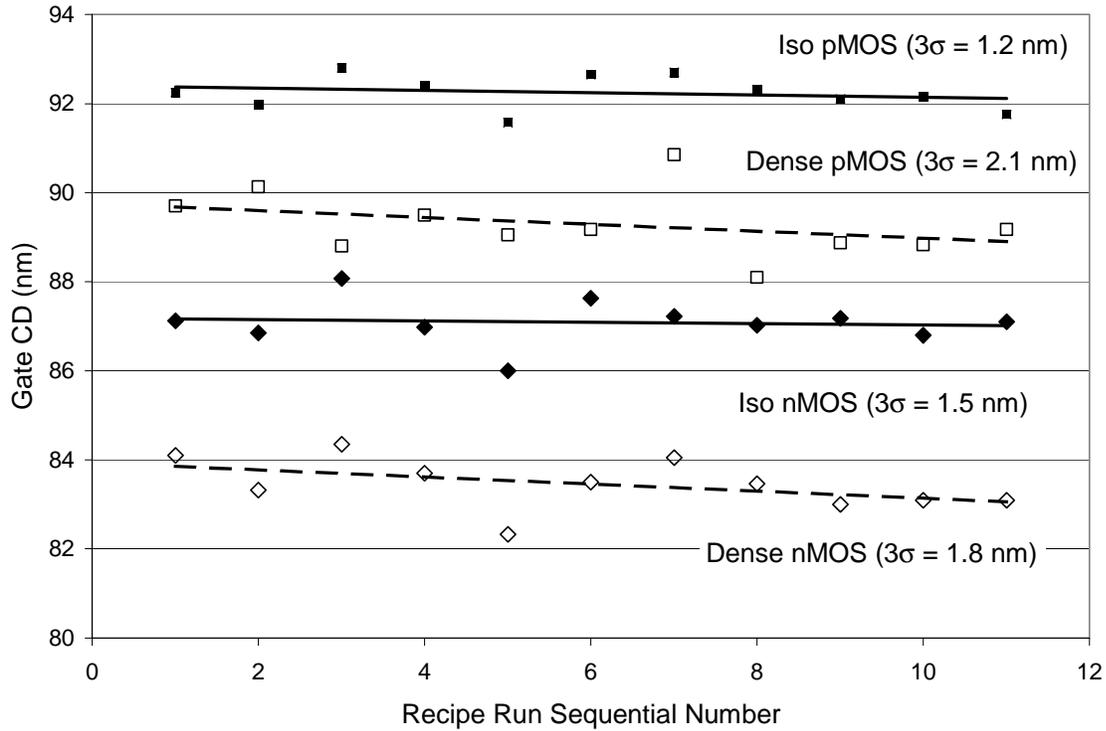
Fig. 2. Short-term dynamic repeatability of CD AFM measurements obtained on isolated and dense polysilicon gates.
