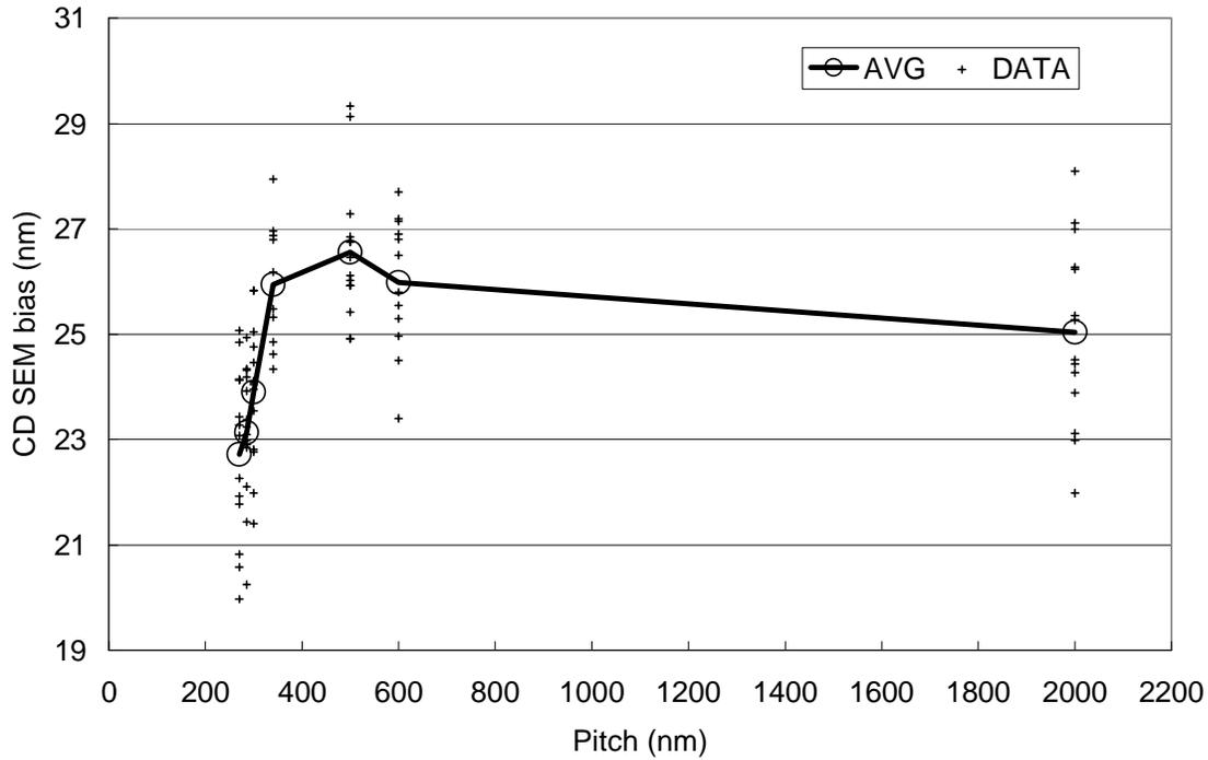
Fig. 6. Sample-to-sample CD SEM bias dependence on polysilicon line pitch. The measured polysilicon lines had smaller height and were patterned using different process compare to the case reported in Fig. 5. CD SEM bias is defined as a difference between mid-derivative line CD by SEM and CD by AFM at 10% of the line height.
