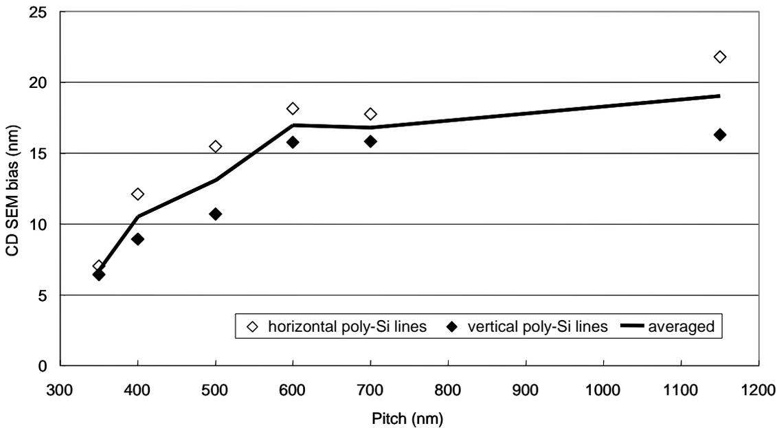
Fig. 5. Sample-to-sample CD SEM bias dependence on polysilicon line pitch. Lines of 2 different orientations on wafer “horizontal” and “vertical” were measured. CD SEM bias is defined as a difference between mid-derivative line CD by SEM and CD by AFM at 10% of the line height.
