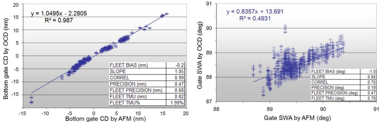
**Figure 3.** The correlation between OCD and reference data for the gate bottom line CD (left) and SWA (right).
