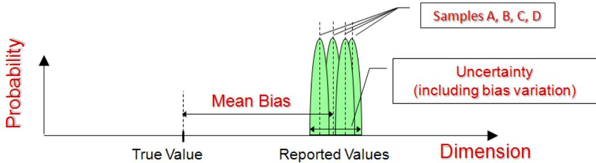
**Figure 1.** Illustration of impact of sample-to-sample bias variation on uncertainty of the measurement [7].
