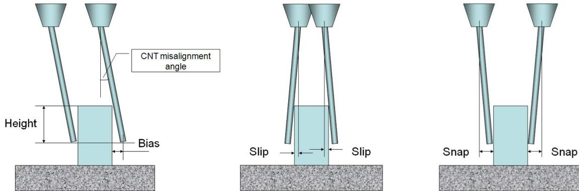
**Figure 6.** Impact of probe misalignment (left), slipping (center) and snapping (right) on diameter measurement uncertainty.
