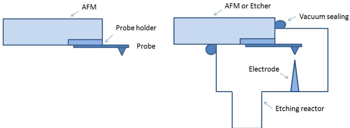
**Figure 10.** Sketch of possible on-tool or off-tool probe cleaning and sharpening solution.
