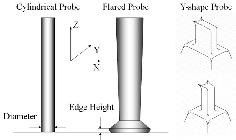
**Figure 5.** Three the most common types of probes used with CDAFM.
