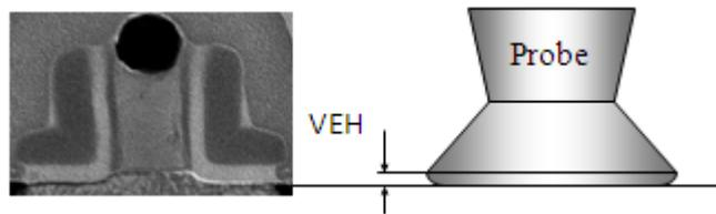
**Figure 8.** Comparison of TEM and CDAFM XZ resolution. Typical vertical edge height (VEH) of flared probes is 5 to 10 nm.
