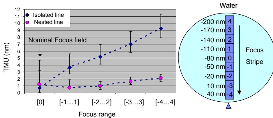
**Figure 1.** The increased CDSEM measurement uncertainty as a function measurand complexity induced by scanner focus.
