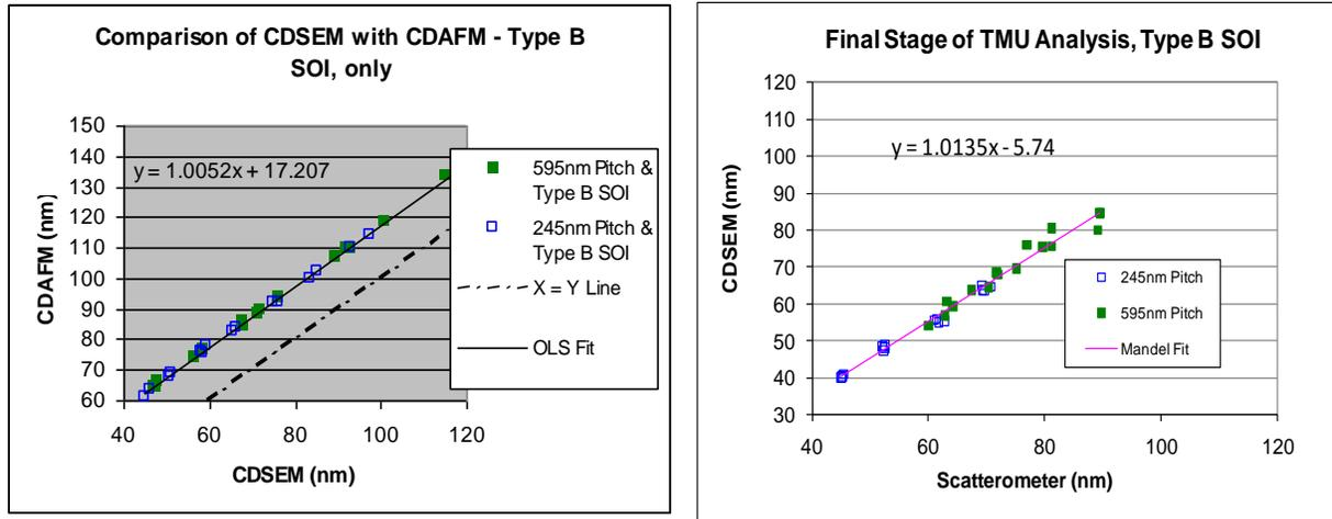
**Figure 2.** An example of using two stages of RM. First stage evaluating the CDSEM with the CDAFM as the RM, and the second stage using the CDSEM as the RM for the scatterometer.
