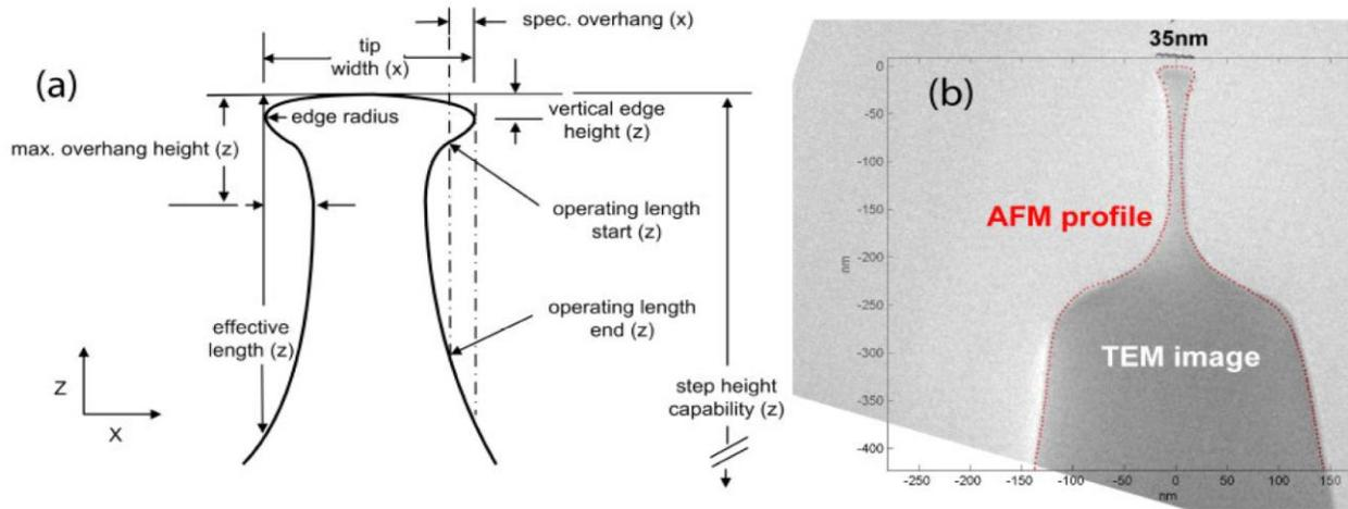
**Figure 11.** (a) shows the important dimensions of a flared probe. (b) shows the superposition of the eroded probe image (red) scan of a characterizer and a TEM image of the same probe. [Dahlen et al ref. 27]
