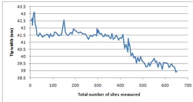
Figure 7. Wear of carbon coated flared probe during interconnect trench CD measurements.
