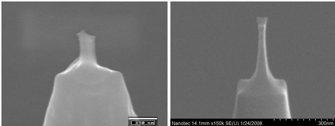
**Figure 9.** SEM images of Y-shape probe. Courtesy of Team Nanotec GmbH (Germany).
