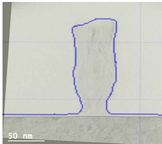
**Figure 12.** Superposition of a reconstructed CDAFM scan and a TEM image of the same sample scanned by the CDAFM. [Dahlen et al ref. 27]
