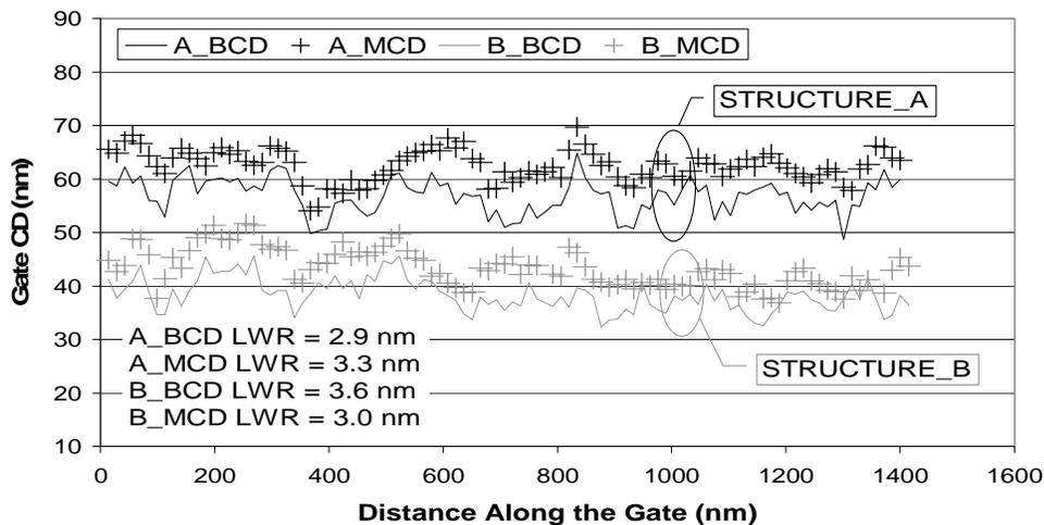
**Figure 19.** The LWR measured for poly-Si lines using CD AFM is shown. The data were collected with rectangular flared probe scanning at  $45^\circ$  to the poly-Si line axis. Both the bottom (BCD) and the middle (MCD) of the line LWR are presented.
