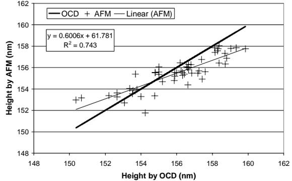
**Figure 12.** Correlation between OCD and AFM data for photoresist line height.
