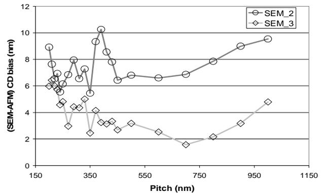
**Figure 10.** Through pitch variation of CD SEM bias observed for 65 nm technology node resist lines on 2 SEM tools.
