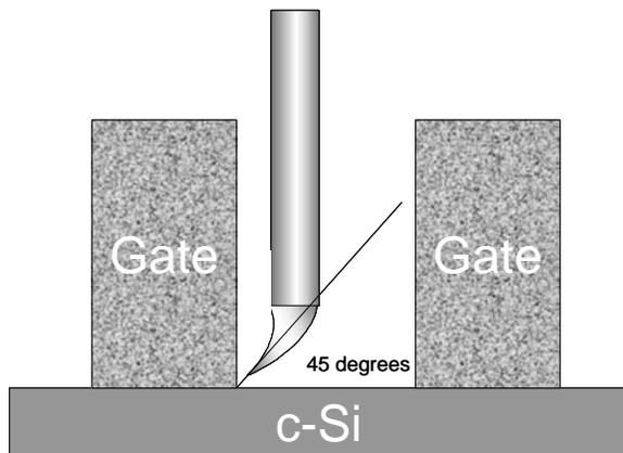
**Figure 23.** New probe design for high resolution AFM.
