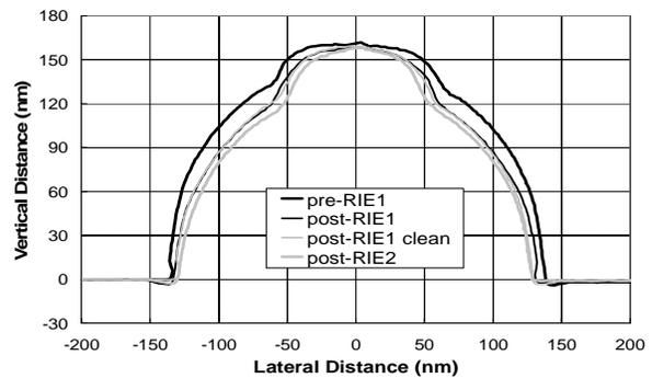
**Figure 18.** The GSS thickness and profile variation measured by CD AFM through IC processing.
