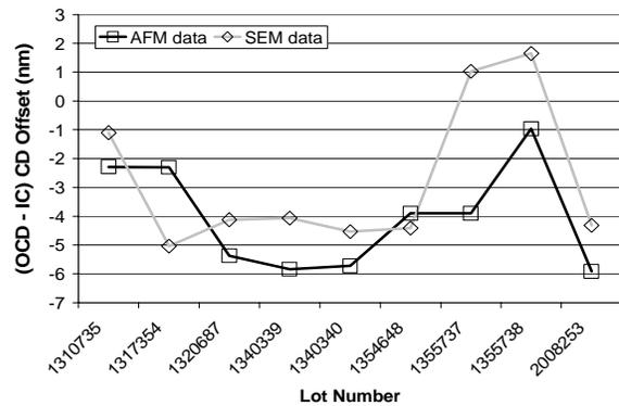
Figure 16. The variation of CD offset between the OCD structure line and the IC transistor gate.
