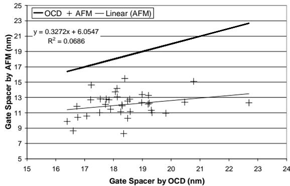
**Figure 17.** Correlation between the GSS thickness measured by OCD and CD AFM.
