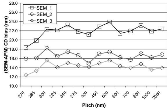
**Figure 8.** Through pitch variation of CD SEM bias observed for 90 nm technology node poly-Si lines on 3 different SEM tools.
