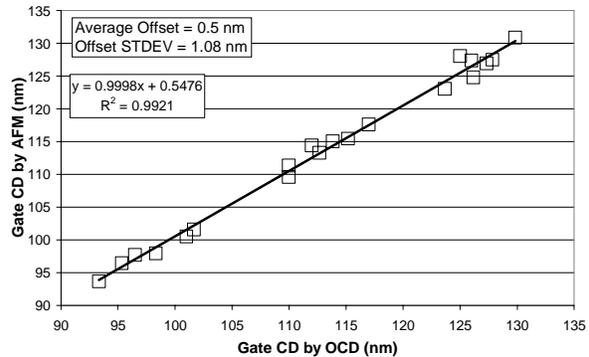
**Figure 14.** Correlation between the lot average poly-Si line CD measured by OCD and CD AFM for 130 nm technology node.
