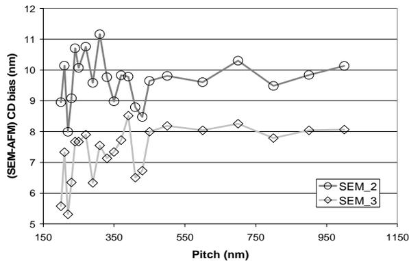
**Figure 9.** Through pitch variation of CD SEM bias observed for 65 nm technology node poly-Si lines on 2 SEM tools.
