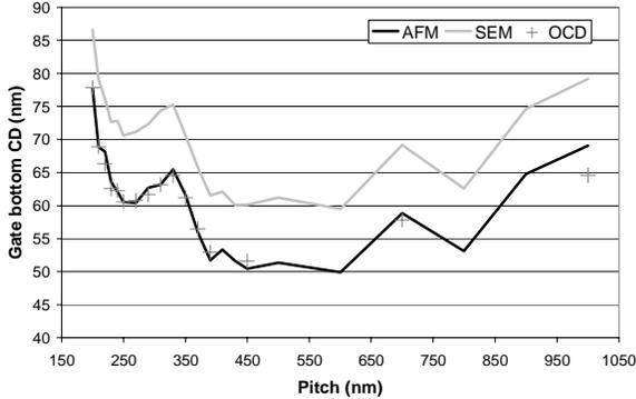
**Figure 11.** Through pitch variation of poly-Si lines CD measured by CD SEM, CD AFM and OCD.
