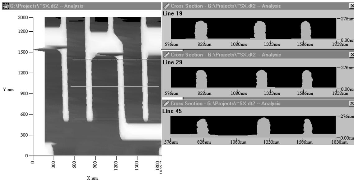
Figure 22. 3D CD AFM image (left) and 3 cross-sections (right) of the gate structure.
