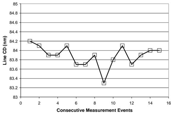
Figure 5. CD AFM dynamic repeatability of 0.7 nm ( $3\sigma$ ) has been demonstrated for line CD measurements.
