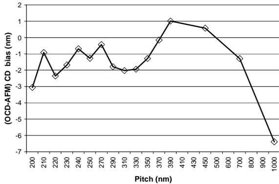
**Figure 13.** Through pitch variation of OCD bias observed for 65 nm technology node poly-Si lines.
