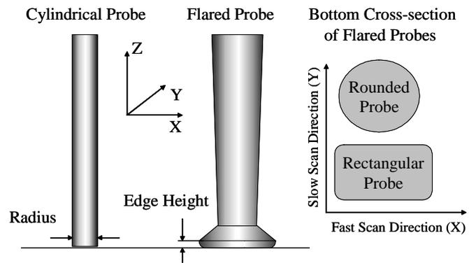
Figure 6. Types of probes used in CD AFM.
