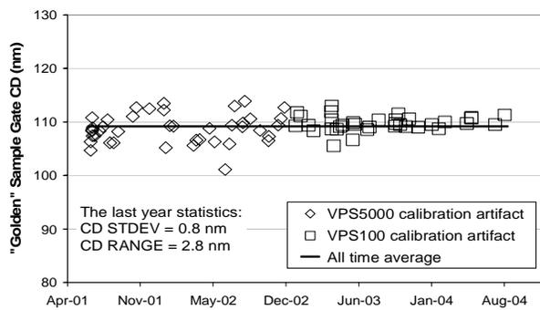
Figure 15. The long-term stability of CD AFM calibration.
