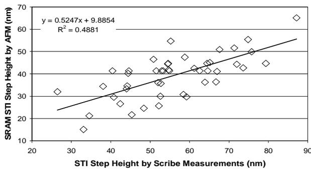
**Figure 7.** Correlation between post-CMP STI topography measured at scribe structure by profilometer and topography measured by AFM in the middle of SRAM array.
