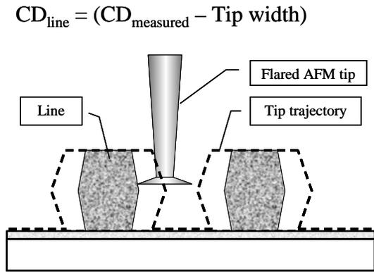
Figure 3. Illustration of CD AFM principle.
